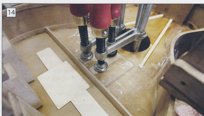
Photo 14. Gluing reinforcing spruce patches in the top. Now I just make one triangular patch, so as not to induce stress points along the grain where a crack might start.
