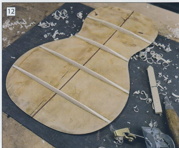
Photo 12. The new braces glued to the back and shaped. When the back is shrunken, you need to add new wood to fit the outline. On this one I put a rosewood strip between the two halves of the back. I usually make the third brace flat to make the back more flexible, but this back was thin and needed more stiffness.
