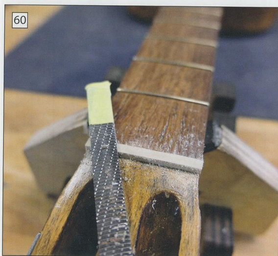
Photo 60. To lengthen the fretboard before intonation measuring, I glue a piece of maple to the end. The height is leveled to the fretboard with a StewMac razor file. The tip of the file is covered with thin plastic tape to protect the fretboard.
