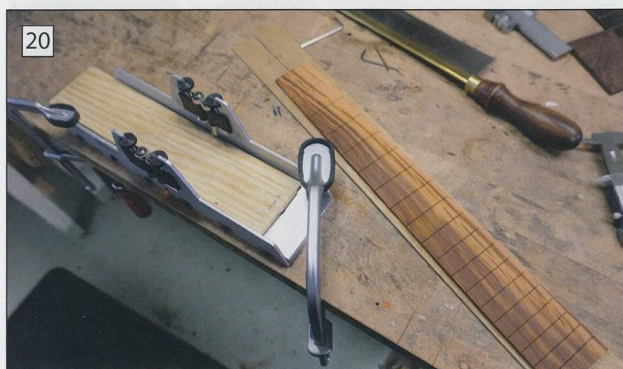
Photo 18. Marking the fret positions using a nice large caliper. I mark with a sharp awl for better precision. When sawing the fret slot, I make sure that the dent from the awl is visible on both sides of the saw.
