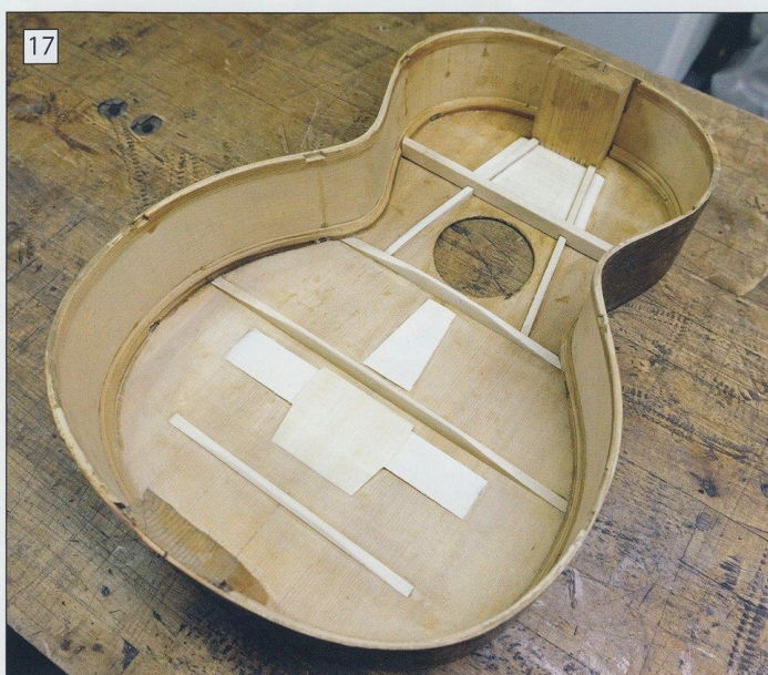
Photo 17. Top braces shaped in a recent ladder bracing with the reinforcement patch under the A-frame, a single patch in the middle, and brace ends tucked in under the lining. The sides of patches in a top should always be thinned out to nothing, or cross more than one grain in the top, to prevent cracks from forming. The main brace under the fretboard is not yet glued.
