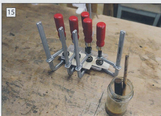
Photo 15. Gluing the pieces of the spruce cross-shaped bridge plate together with hot hide glue.
