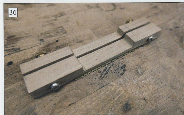
Photo 45. I glue a wooden shim on the underside of the segmented saddle to make it stronger. This also gives me another opportunity to adjust the height of the saddle if it turned out to be too low.
